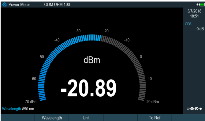
Optical power measurement with optical power sensor.
